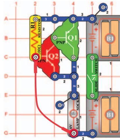
**OBJECTIVE:** To compare transistor circuits.
