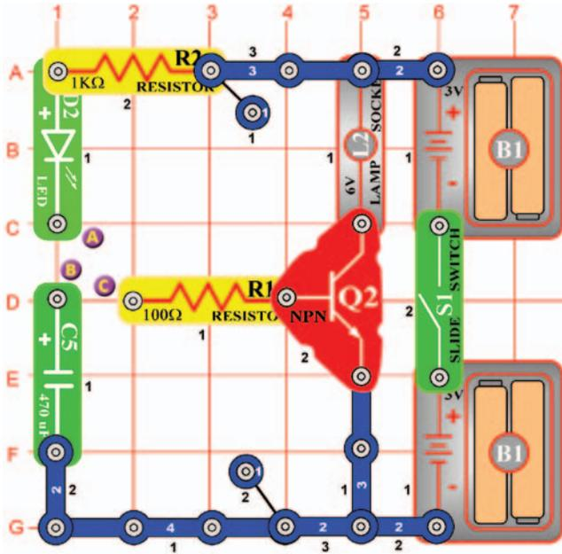
Turn the slide switch (S1) on and connect points A & B with a 2-snap wire. The green LED (D2) will flash and the 470µF capacitor (C5) will be charged with electricity. The electricity is now stored in the capacitor. Disconnect points A & B. Connect points B & C and there will be a flash from the 6V lamp (L2).
