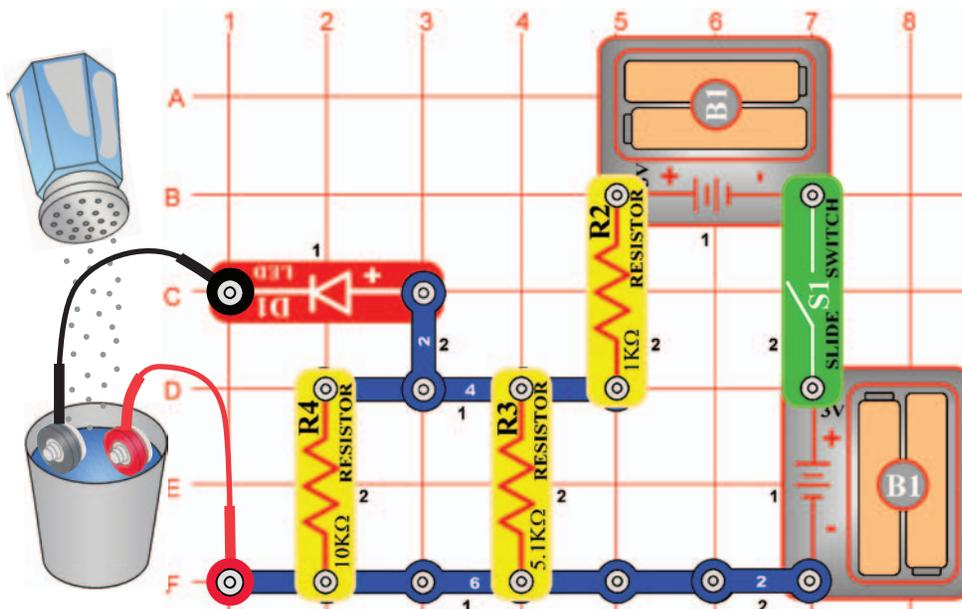
Place the jumpers in a cup of water as in the preceding project; the LED (D1) should be dimly lit. Slowly add salt to the water and see how the LED brightness changes, mix it a little so it dissolves. It will slowly become very bright as you add more salt. You can use this bright LED condition as a saltwater detector! You can then reduce the LED brightness by adding more water to dilute the salt.
