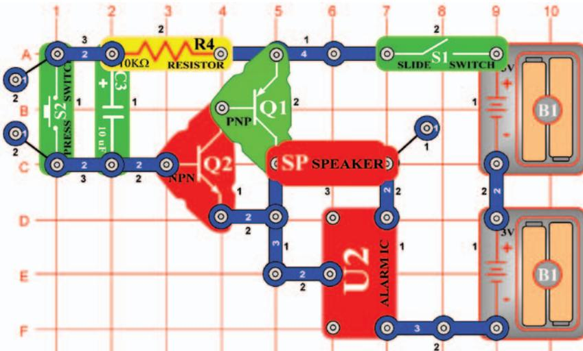
Turn on the slide switch (S1), then press and release the press switch (S2). You hear a siren that slowly fades away and eventually goes off. You can modify this circuit to make machine gun or ambulance sound instead like in the other projects. You can also replace the 10µF capacitor (C3) with the 100µF (C4) or 0.1µF (C2) to greatly slow down or speed up the fading.
