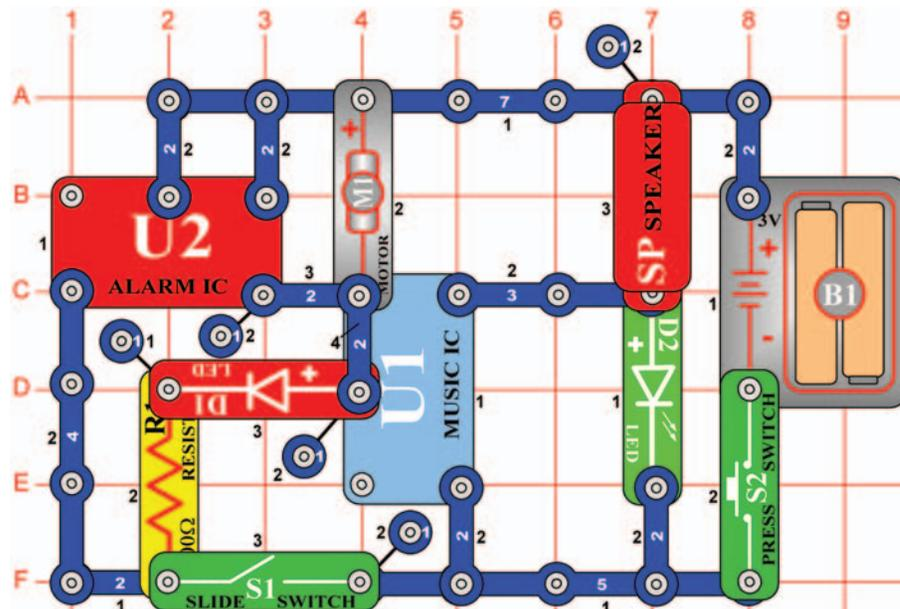
Build the circuit shown on the left. Place the fan onto the motor (M1). In the circuit, the alarm IC (U2) and the music IC (U1) are connected together. The sounds from both IC's can be played at the same time. Press the press switch (S2). The music IC plays and the green LED (D2) lights. Now turn on the slide switch (S1) and press the press switch again. You should hear the sounds from both IC's playing. As the alarm IC plays, it also drives the fan and the red LED (D1).
