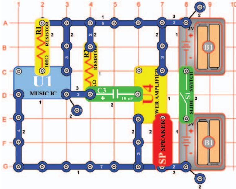
Build the circuit and turn on the slide switch (S1). You will hear loud music, since the sound from the music IC (U1) is amplified by the power amplifier IC (U4). All radios and stereos use a power amplifier.
