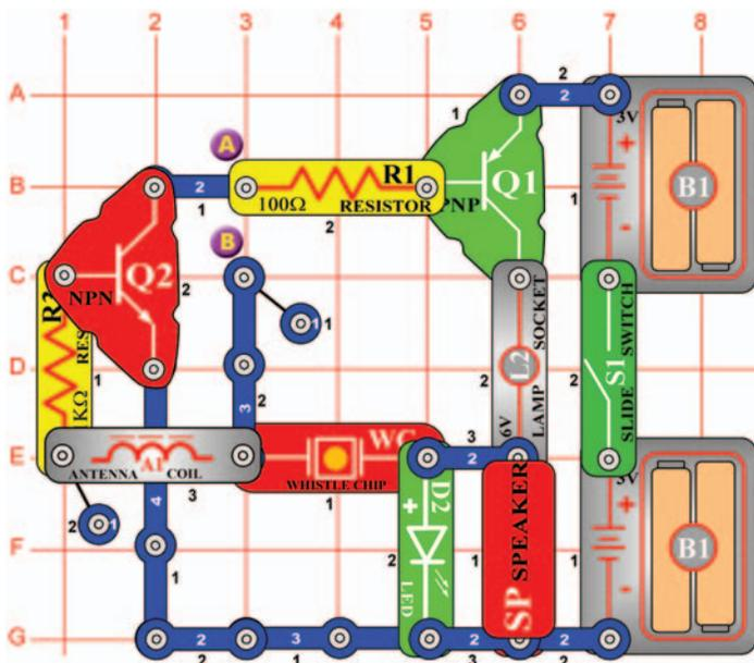
Turn on the slide switch (S1) and place your finger across points A & B. The speaker (SP) will output a tone and the LED (D2) will flash at the same frequency. Your finger acts as a conductor connecting points A & B. When a person is lying, one thing the body starts to do is sweat. The sweat makes the finger a better conductor by reducing its resistance.
