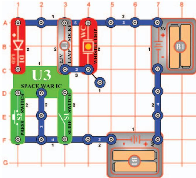
**OBJECTIVE:** To show how sound can turn "ON" an electronic device.
