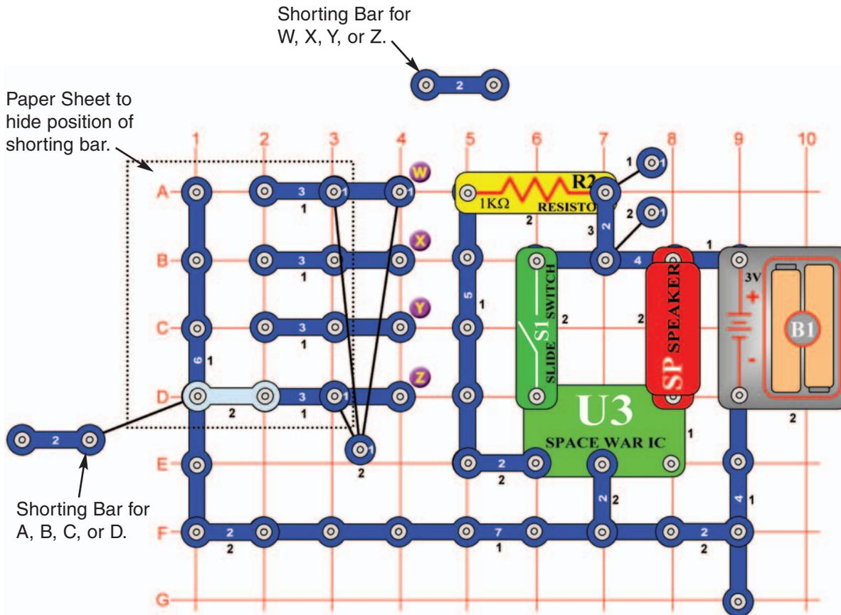
Build the circuit shown on the left. It uses two (2) 2-snap wires as shorting bars.
