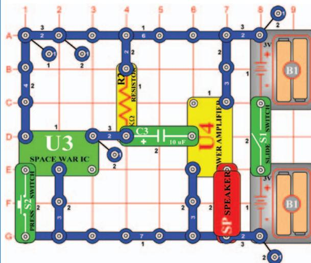
Build the circuit, turn on the slide switch (S1), and press the press switch (S2) several times. You will hear loud space war sounds, since the sound from the space war IC (U3) is amplified by the power amplifier IC (U4). Nearly all toys that make sound use a power amplifier of some sort.
