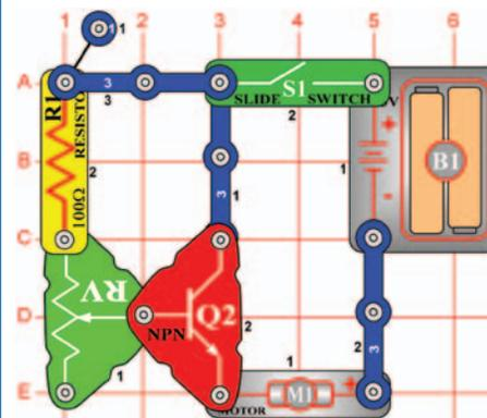
**OBJECTIVE:** To compare transistor circuits.
