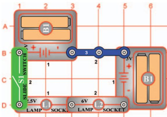
Turn on the slide switch (S1) and both lamps (L1 & L2) will light. If one of the bulbs is broken then neither will be on, because the lamps are in series. An example of this is the strings of small Christmas lights; if one bulb is damaged then the entire string does not work.
