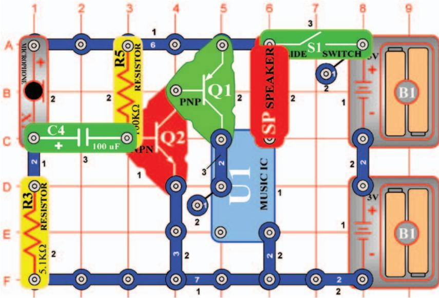
**OBJECTIVE:** To turn off a circuit by blowing on it.
