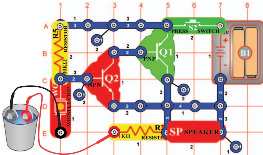
Build the circuit at left and connect the two (2) jumpers to it, place the loose ends of the jumpers into an empty cup (without them touching each other). Press the press switch (S2) - nothing happens. Add some water to the cup and an alarm will sound. Add salt to the water and the tone changes.
