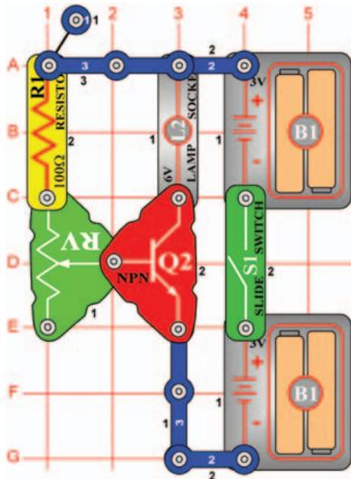
**OBJECTIVE:** To compare transistor circuits.
