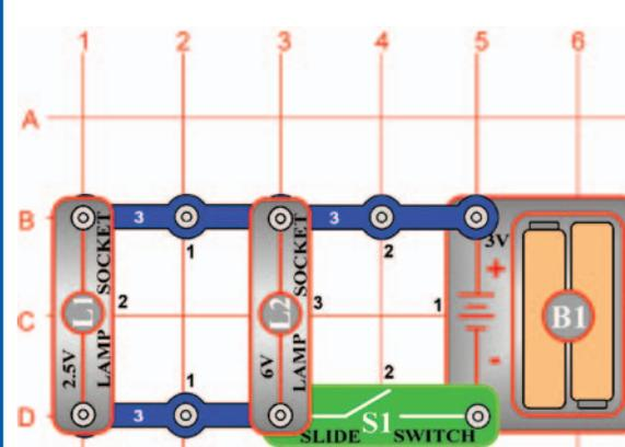
Turn on the slide switch (S1) and both lamps (L1 & L2) will light. If one of the bulbs is broken then the other will still be on, because the lamps are in parallel. An example of this is most of the lights in your house; if a bulb is broken on one lamp then the other lamps are not affected.
