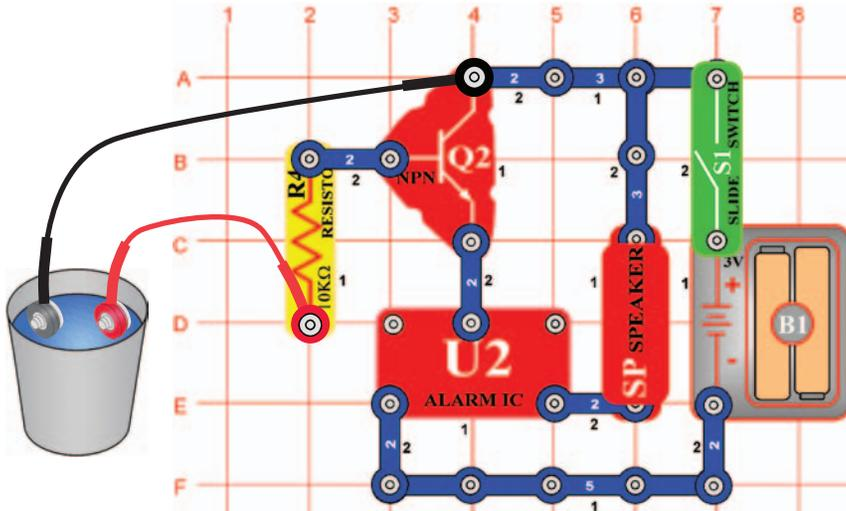
Build the circuit on the left and connect the two (2) jumpers to it, place the loose ends of the jumpers into an empty cup (without them touching each other). Turn on the slide switch (S1) - nothing happens. This circuit is designed to detect water and there is none in the cup. Add some water to the cup - an alarm sounds!
