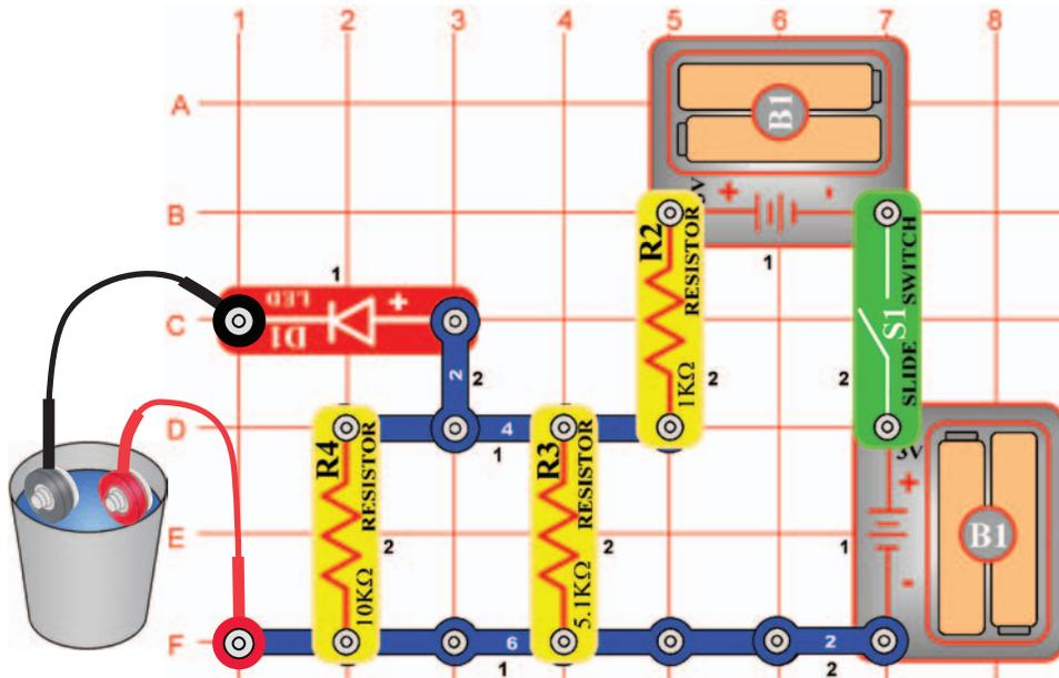
Build the circuit at left and connect the two jumpers to it, but leave the loose ends of the jumpers lying on the table initially. Turn on the slide switch (S1) - the LED (D1) will be dark because the air separating the jumpers has very high resistance. Touch the loose jumper ends to each other and the LED will be bright, because with a direct connection there is no resistance separating the jumpers.
