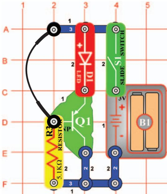
**OBJECTIVE:** To build a transistor light alarm.
