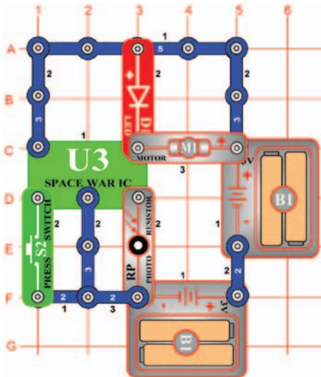
**OBJECTIVE:** To vary the speed of a fan activated by light.
