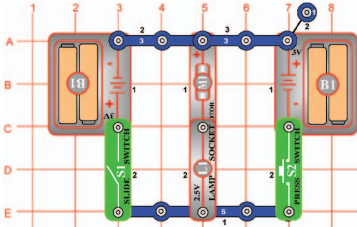
**OBJECTIVE:** To show how voltage polarity affects a DC motor.
