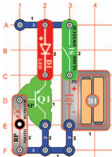
**OBJECTIVE:** To compare transistor circuits.
