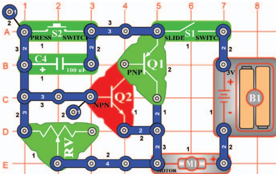
**OBJECTIVE:** To build a circuit that controls how long the fan is on.
