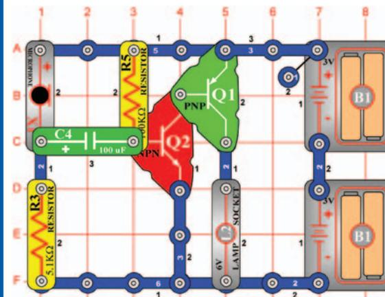
Install the parts. The lamp (L2) will be on. It will be off as long as you blow on the mic (X1). Speaking loud into the mic will change the brightness of the lamp.
