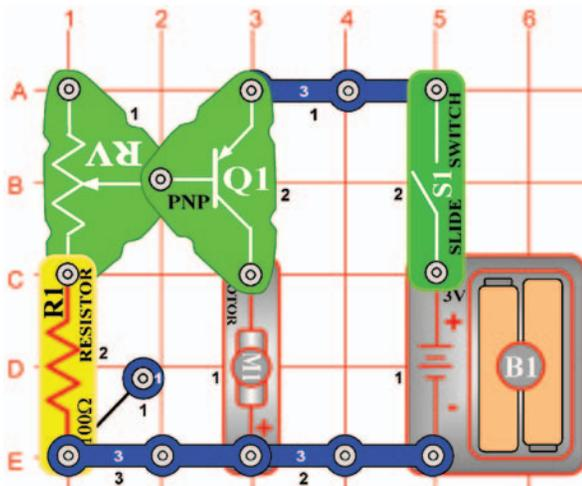
**OBJECTIVE:** To adjust the speed of a fan.
