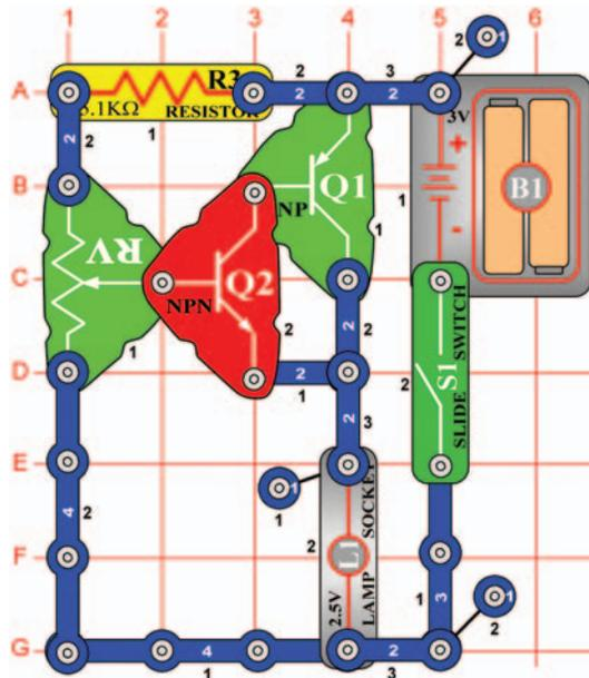
Here is a combination with two transistors. This combination increases the amplifying power. By changing the resistance, the current at the base of the transistor is also changed. With this amplifying ability of the combination, there is a greater change of current to the lamp (L2). This changes the brightness.
