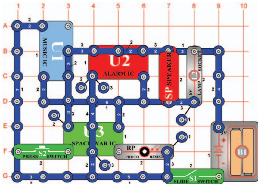
Build the circuit shown. Turn it on and press the press switch (S2) several times and wave your hand over the photoresistor (RP) to hear the full symphony of sounds that this circuit can create. Have fun!
