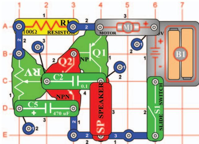
Build the circuit on the left. Turn on the slide switch (S1) and move the setting on the adjustable resistor (RV) across its range. You hear screaming sounds and the fan spins.
