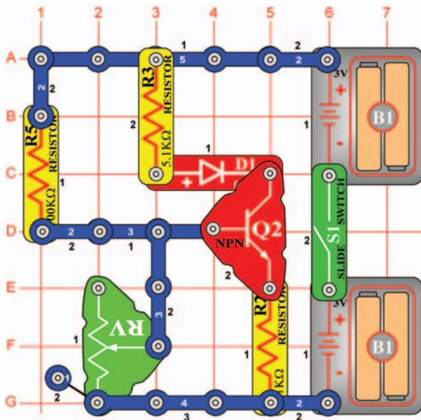
Turn on the slide switch (S1) and move the adjustable resistor (RV) control lever across its range. When the lever is all the way down the LED (D1) will be off, as you move the lever up it will come on and reach full brightness.
