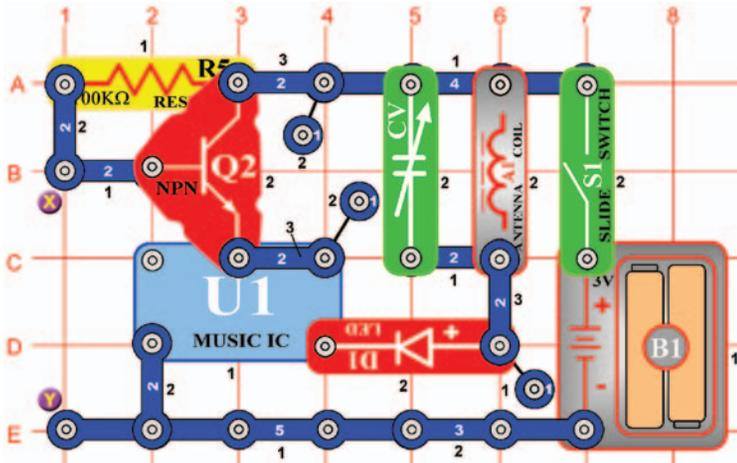
You need an AM radio for this project. Build the circuit on the left and turn on the slide switch (S1). Place it next to your AM radio and tune the radio frequency to where no other station is transmitting. Then, tune the adjustable capacitor (CV) until your music sounds best on the radio. Now connect a jumper wire between X and Y on the drawing, the music stops.
