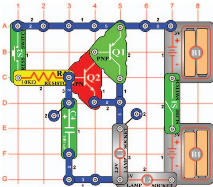
Turn on the slide switch (S1) and press the press switch (S2). The lamps (L1 & L2) turn on slowly, but stay on for a while after you release the press switch.
