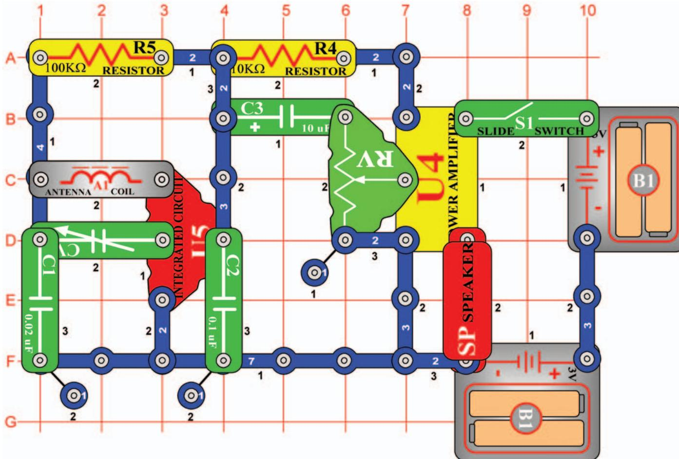
When you turn on the slide switch (S1), the integrated circuit (U5) should amplify and detect the AM radio waves all around you. The variable capacitor (CV) can be tuned to the desirable station. Varying the adjustable resistor (RV) will make the audio louder or softer. The power amplifier IC (U4) drives the speaker (SP) to complete the AM radio project.
