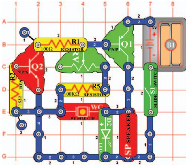
Build the circuit, turn it on, and move the setting on the adjustable resistor (RV). It makes a loud, annoying whine sound. The green LED (D2) appears to be on, but it is actually flashing at a very fast rate.
