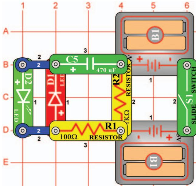
Build the circuit (be sure the positive (+) side of the capacitor is towards the left) and turn on the slide switch (S1). The green LED (D2) will flash brightly as the 470µF capacitor (C5) charges up and then becomes dim but will not be off. When you turn off the slide switch, the red LED (D1) is initially bright, but goes dim as the capacitor discharges itself through it.
